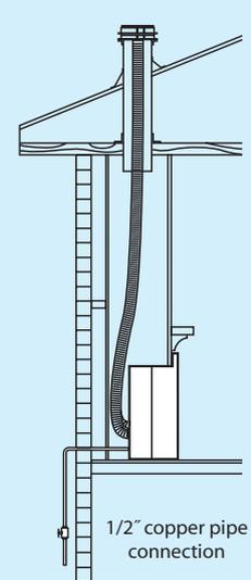
Two fully flexible flues are included. The first is a 50mm diameter pipe to expel gas fumes, whilst the second 60mm diameter flue brings fresh air into the firebox chamber.
